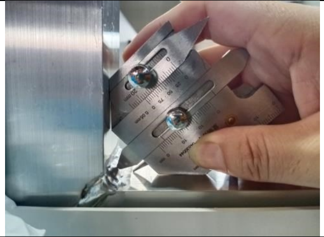
8. The reinforcement in the middle were welding from 3 sides, the welding was done with gap
