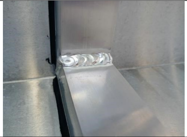
8. The reinforcement in the middle were welding from 3 sides, the welding was done with gap
