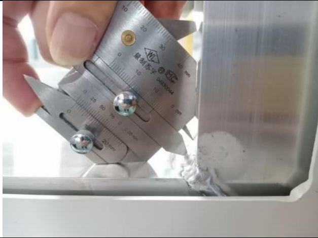
8. The reinforcement in the middle were welding from 3 sides, the welding was done with gap
