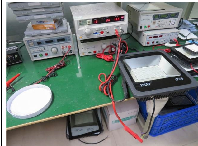
Earth continuity test
