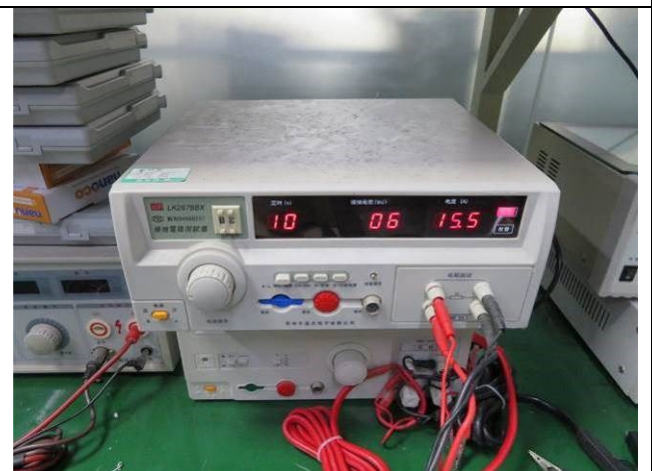
Earth continuity test
