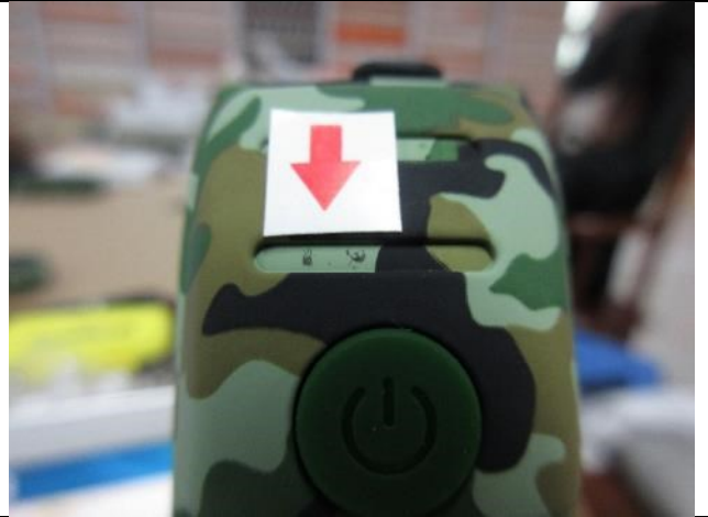
Poor water transfer printing - Minor
