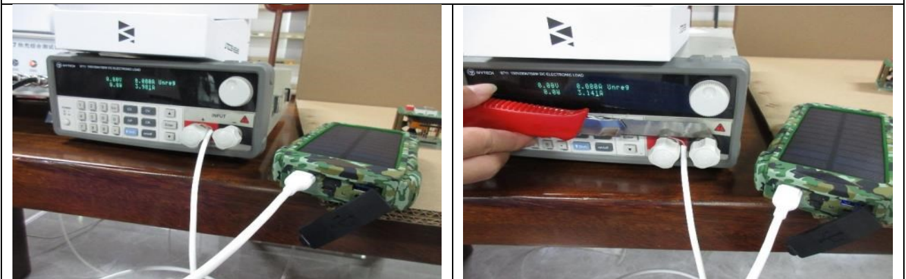
Overloading current protective test
