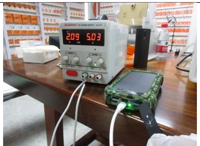
Output current loading test
