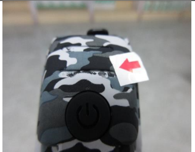
Poor water transfer printing - Minor
