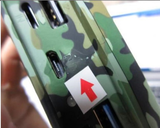
Poor water transfer printing - Minor
