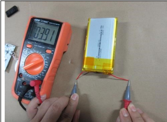
The battery voltage check
