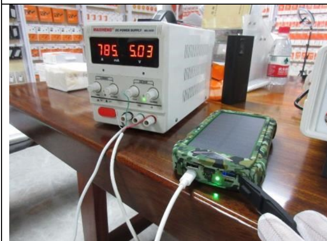
Output current loading test
