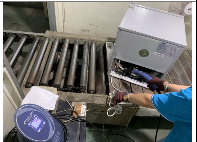
Refrigerating fluid leakage test
