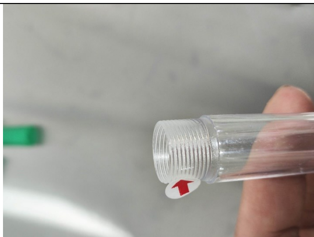
Cracked case-major issue
