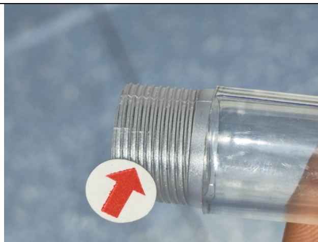
Cracked case-major issue
