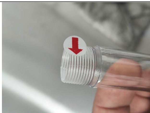
Cracked case-major issue
