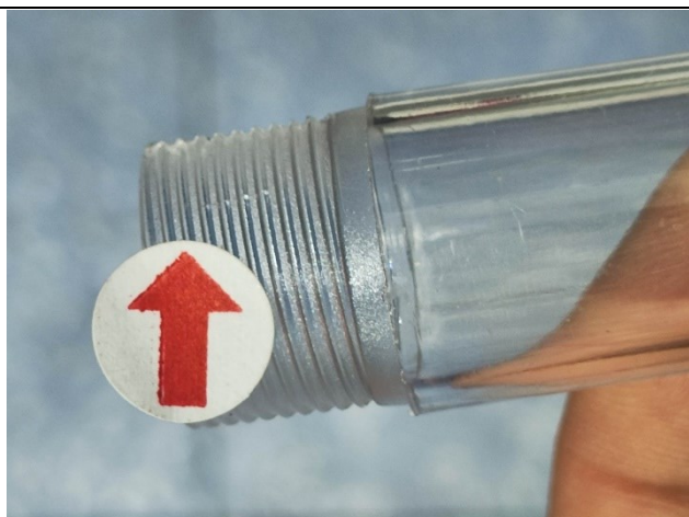
Cracked case-major issue
