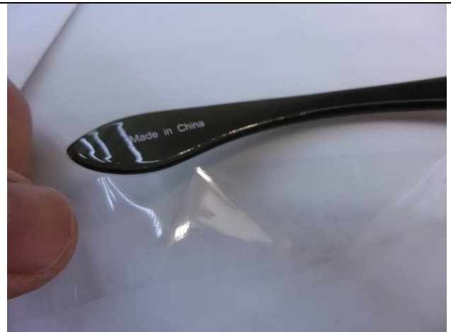
3M tape testing on coating
