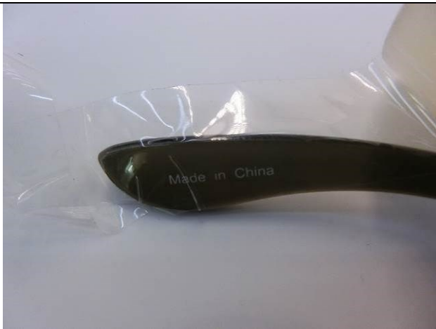
3M tape testing on coating
